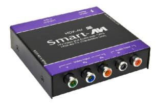
Use a single CAT5 to broadcast high resolution HDTV Video, Stereo Audio, up to 1000ft away.
