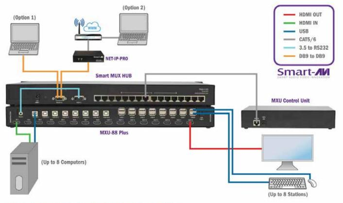
Transparent USB 2.0 Switching. Access to any USB Device for Any Station.
