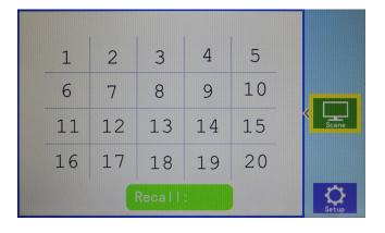
The Scene page on the front panel allows for easy playing of preconfigured layouts. Simply press the number corresponding to the desired layout, then press 'Recall' to play the desired layout.
