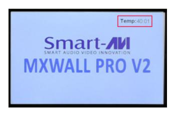
The MXwall Pro V2 front panel displays the temperature of the unit in degrees Celsius in order for users to monitor and prevent overheating.
