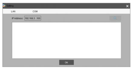
3. To connect to the unit over RS232, select 'COM'. Enter the correct COM port and Baud Rate, and then press 'Connect' and then 'OK'.
